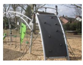
The curved climbing wall is made of a steel frame supported Ekogrip® panel with unique designed climbing cleats. The Ekogrip® panel consist of a 15mm thick PE base with 3 mm top-layer of rubber with a non-skid effect.
