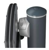
The connectors are made of die-cast aluminum specially alloyed for outdoor environments and with a lead content below 100ppm. The connectors are attached to the posts by stainless steel screws and well protected against corrosion by special designed zinc washers. Extremely strong and no change of corrosion.
