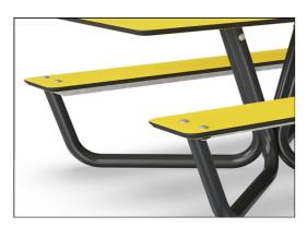
All boards are made of High Pressure Laminate HPL with a .7 in. thickness according to EN 438-6 and has a nonskid surface texture. The multilayer construction makes the boards durable and suited for outdoor use, with a high resistance to impacts, scratches, fire, water and humidity, as well as high UV stability.
