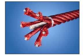
Corocord ropes of UV-stabilized PES rope strands with inner steel cable reinforcement. The polyester yarn is made from +95% post-consumer materials and is inductively melted onto each strand. PES has high strength with excellent resistance to abrasion and UV radiation. The ropes are connected by stainless steel S-Clamps which are pressed around the rope which results in a durable and vandalism solution/20024
