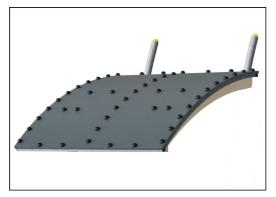
Roof is made of a steel frame supported Ekogrip® panel. The Ekogrip® panel consist of a 15mm thick PE base with 3 mm top-layer of rubber.
