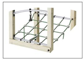
Corocord ropes of UV-stabilized PES rope strands with inner steel cable reinforcement. The polyester yarn is made from +95% postconsumer materials and is inductively melted onto each strand. PES has high strength with excellent resistance to abrasion and UV radiation. The rope loops are assembled by aluminum connectors.
