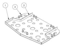
A 5 mm hot-dip galvanised carbon steel plate to the frame.
