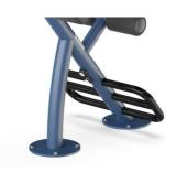
All Steel components are made from carbon steel, with a hot-dip galvanized surface according to ISO1461, and a powder coating corrosion class C3 according to ISO12944-2. Lead content for surfaces is below 90ppm, and below 100ppm for base material.
