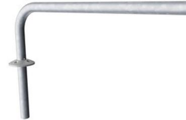
Handrail intended as grips during exercises are made of hot-dip galvanised steel  $\varnothing 38\text{mm}$ , a great diameter for a good grip and to support the wrist. The height of the handrail is 940mm from the top of the HPL plate. The distance between the rails is 900mm.
