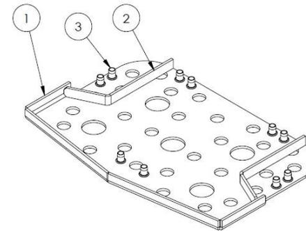
A 5 mm hot-dip galvanised carbon steel plate must be moulded inside the SBR to offer optimal stability and optimize the mounting of the step to the frame.
