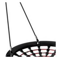
Ropes are made of UV-stabilized PA with inner steel cable reinforcement. The rope is induction treated in order to create a strong connection between steel and rope which leads to good wear resistance.
