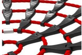
Rope loops of the seat are made of single braided 16 mm PES ropes. The polyester yarn is made from +95% post-consumer materials and is inductively melted onto each strand. PES has high strength with excellent resistance to abrasion and UV radiation. The rope loops are connected by nylon (PA6) connectors.
