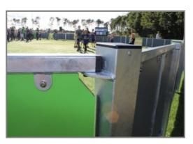
The HDPE panels are connected with M8 stainless steel bolts to  $42.5 \times 40 \times 3$ mm welded flanges. These connections are not visible from the inside and create a strong and safe connection.
