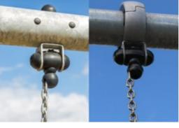
The swing hangers are made of high-quality UV-stabilised nylon (PA6) housing with integrated lifetime sealed ball bearings. The adjustable chains are fixed by a stainless steel hook with a theft-proof snake-eye bolt which is manufactured within an anti-twist house. All seats are fixed with two chains and are available with either standard or anti-wrap suspension.
