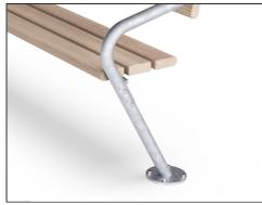
The steel surfaces are hot dip galvanized inside and outside with lead free zinc. The galvanization has excellent corrosion resistance in outdoor environments and require low maintenance. Painted steel parts are hot dip galvanized before powder coating.
