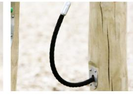
Ropes are made of UV-stabilised PA with inner steel cable reinforcement. The rope is induction treated to create a secure connection between steel and rope, which leads to excellent wear resistance.
