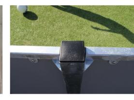
The posts are made of 80 x 80 x 3mm profile with horizontally, 6mm welded flanges. This will enable easy installation and strong construction. The low-density polyethylene post caps are attached with blind rivets.
