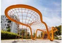
The steel surface of these bent steel pipes are painted with one basic layer and one top layer of lead-free colour material. The paint has excellent corrosion resistance and can be easily maintained.
