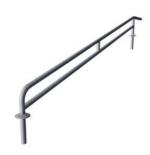
The railing height is 930mm and the distance between the railing is 900mm The material used for the railing is hot-dip galvanised steel ø38 mm, a great diameter for a good grip and wrist support.
