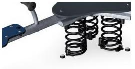
KOMPAN's springs are manufactured from highquality spring steel. The springs are cleaned by phosphating before being painted with epoxy primer and polyester powder coating. The springs are fixed by unique anti-pinch fittings for maximum safety and longevity.
