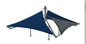
Sails of commercial 95 high-density PE knitted specially for sun-shade structures. The sails are treated with UV stabilisers to ensure longevity. The sails are supported by a hot-dip galvanised steel frame and tightened by stainless-steel devices.
