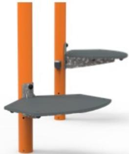
The top plate for the jumping platform is made of Ekogrip® panels that consist of a 15 mm polyethylene bottom layer, with a 3 mm top-layer of thermoplastic rubber with a non-skid effect for safe jumping exercises under all-weather circumstances.
