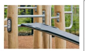
The surface is made of Ekogrip<sup>™</sup> panels, consisting of 15mm polyethylene with a 3mm top-layer of thermoplastic rubber. The Ekogrip™ panels have a non-skid effect for comfortable and safe training at all weather circumstances.
