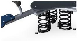
KOMPAN Springs are made of high quality spring steel according to EN10270. The springs are cleaned by phosphating before they are painted with an epoxy primer and a polyester powder coating as top finish. The springs are fixed by unique anti pinch fittings for maximum safety and long lifetime.
