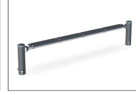
The steps are made of High Pressure Laminate HPL with a thickness 17,8mm and non skid surface texture according to EN 438-6. KOMPAN HPL has high wearing strength to ensure long lifetime in all climates.
