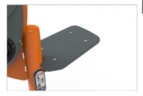
Seat is made of Ekogrip™ panel that consist of a 15mm thick PE base with 3 mm top-layer of soft rubber with a non-skid effect.
