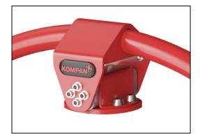
The rocking movement is controlled by a heavy duty scaled rubber torsion spring element. The rubber element ensures a damped movement up and down.
