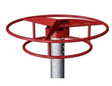
The upper twin ring has a base of hot dip galvanization and a powder coated top finish. This provides an ultimate corrosion resistance in all climates around the world. Steps are made of PUR. It retains their properties in the temperature range of -30°C to 60°C. Step is stabilized to a maximum without use of heavy metal stabilities.
