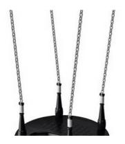
The double steel yoke suspension provides the unique parallel movement of the seat. The swing hangers are made of high quality UV stabilised nylon (PA6) housing with integrated lifetime sealed ball bearings. The height adjustable chains are fixed by a stainless steel hook with theft proof snake eye bolt in a turn able anti twist housing.
