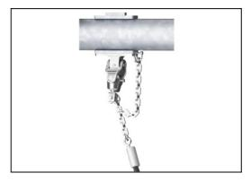
KOMPAN's swing hangers are heavy-duty and designed with stainless steel and anti-twist functions. The hangers attach to the cross beam on a welded bracket with two bolts. The bearings are embedded with silicone lubricant and need no further lubrication; ensuring low maintenance.
