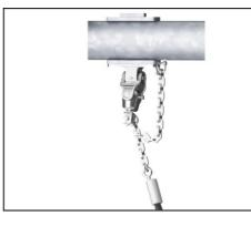
KOMPAN's swing hangers are heavy-duty and designed with stainless steel and anti-twist functions. The hangers attach to the cross beam on a welded bracket with two bolts. The bearings are embedded with silicone lubricant and need no further lubrication; ensuring low maintenance.
