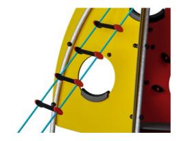
Ropes are made of UV-stabilised PA with inner steel cable reinforcement. The rope is induction treated in order to create a strong connection between steel and rope which leads to good wear resistance.
