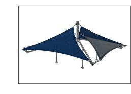
Sails of commercial 95 high density PE knitted specially for sun-shade structures. The sails are treated with UV stabilizers to ensure a long lifetime. The sails are supported by a hot dip galvanised steel frame and tightened by stainless steel devices.
