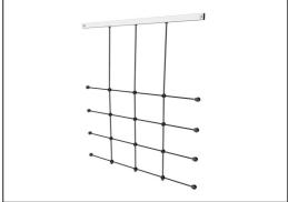
Climbing nets are made of UV-stabilised PP rope with inner steel cable reinforcement. The rope is induction treated to obtain maximum fixation between steel and rope which provides excellent wear and tear resistance. All rope connectors are made of 100% recyclable PA material.
