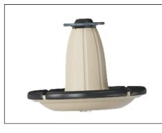
The central part of the Boogie Spinner is made of recyclable polyethylene (PE) made from 33% post-consumer materials and is rotomoulded in one piece with integrated metal thread bushings and water drain holes to ensure high durability in all climates around the world.
