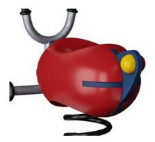
The seat is made of recyclable PE and molded in one piece with a minimum 5mm wall thickness. PE has high impact resistance across a wide temperature span which ensures vandal resistance in all locations.
