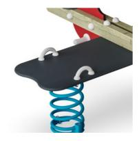
Foot support is made of HPL with a thickness of 17,8mm with a very high wearing strength and a unique KOMPAN nonskid surface texture.
