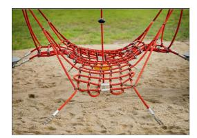
Ropes are made of UV-stabilized PES rope strands with inner steel cable reinforcement. The polyester wrapping is inductively melted onto each strand to ensure excellent wear and tear resistance.
