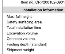
1'3" Safety surfacing area 316ft<sup>2</sup> Total installation time 6.7 hours 1.35yd3 1.11yd3 Footing depth (standard) 2'11" 463lbs In-ground Anchoring options Surface **Warranty Information**
