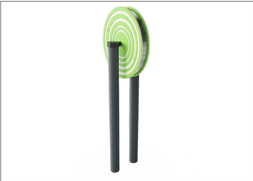
Round Ø100mm posts of extruded aluminum with powder coated top finish in black color and High-Density Polyethylene HDPE post cap
