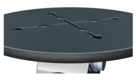
The ø414mm top plate is made from 15mm Ekogrip®, a 15mm PE plate with a 3mm toplayer of thermoplastic rubber with non-skid effect. The height is 217mm and the range of motion is  $+/-90^{\circ}$ , with a EPDM rubber stop at each end.
