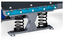
KOMPAN Springs are made of high quality spring steel according to EN10270. The springs are cleaned by phosphating before they are painted with an epoxy primer and a polyester powder coating as top finish. The springs are fixed by unique anti pinch fittings for maximum safety and long lifetime.
