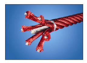
Ropes of UV-stabilized PES rope strands with inner steel cable reinforcement. The polyester yarn is made from +95% post-consumer materials and is inductively melted onto each strand. The ropes are highly wear-and vandalism-resistant and can be replaced at site if needed.
