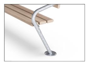
The steel surfaces are hot dip galvanized inside and outside with lead free zinc. The galvanization has excellent corrosion resistance in outdoor environments and require low maintenance. Painted steel parts are hot dip galvanized before powder coating.
