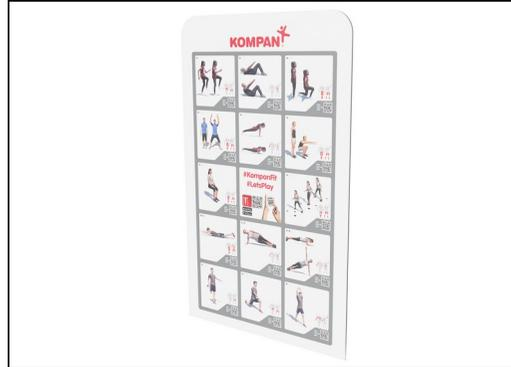
High-quality polycarbonate with a thickness of 8mm. The graphic prints are added by a unique multi-layer print process where the inner layer is the image and outer transparent layer functions as protection. Both PC panel and the water-based lacquer are UV stabilized to prevent fading.
