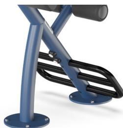
All Steel components are made from carbon steel, with a hot-dip galvanized surface according to ISO1461, and a powder coating corrosion class C3 according to ISO12944-2. Lead content for surfaces is below 90ppm, and below 100ppm for base material.
