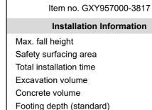
Installation Information 150 cm 69.4 m<sup>2</sup> 3.0 1.20 m<sup>3</sup> 0.80 m<sup>3</sup> Footing depth (standard) 120 cm Shipment weight 183 kg Anchoring options In-ground Surface
