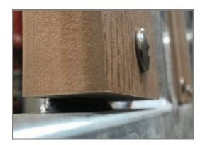
The Wood Plastic Composite panels are made of 100% recycled fibre/wood powder and High-Density Poly Ethylene (HDPE). With the dimensions of 860 x 110 x 30mm the boards are solid.
