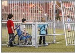
The wheelchair entrance is constructed of 80 x 80 x 3mm post with Ø 48mm tube and two stainless steel 16mm hinges. The opening is 95cm wide and 112cm long, which allows wheelchair users to enter the MUGA with ease.
