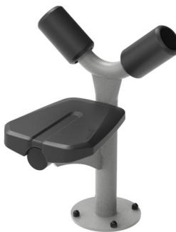
The seat is made of Polyurethane Rubber and has a steel insert plate that is electro-galvanized. The steel plate connects the seat to the frame. This construction makes the seat extremely durable against wear & tear and still very comfortable for a great user experience. The seat is positioned at a height of 46 cm, a comfortable height that makes the transfer from a wheelchair easy.
