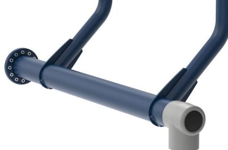
The input shaft is Ø101,3 x 2,9mm S355 Hot Dip Galvanized and Powder-coated steel. The bearing house is Caste Aluminum (EN AB-44100 / EN AB-AlSi12(a)) with self-aligning sealed ball bearings. An extremely strong and durable construction
