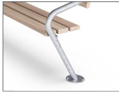
Steel internal surfaces are hot-dip galvanised, and the outside surfaces are lead and zinc free. Galvanisation has excellent corrosion resistance within outdoor environments and requires very little maintenance. Painted steel parts are hotdip galvanised and then powder coated.
