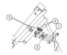
The steel cable three is tensioned by a specially designed device. By turning the handle, the steel cable can be tensioned safety. After tensioning the cable is locked by three clamps two. The tensioning device can also be used for adjustment during annual inspections.
