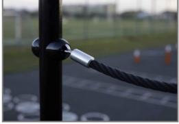
Ropes are made of UV-stabilised PA with inner steel cable reinforcement. The rope is induction treated in order to create a strong connection between steel and rope, which leads to excellent wear resistance.
