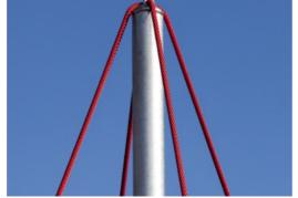
In the center of the net is the mast, made of high quality seamless steel. The structure of the mast as an oscillating support is statically favorable and equalizes the oscillations in the net. The masts are hot dip galvanized as standard, with the design option of additional powder coating.
