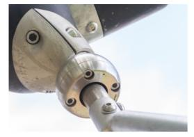
Bearing systems in heavy duty design in a maintenance free construction. All steel bearings are fully closed and lifetime lubricated.
