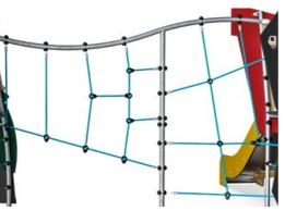
Climbing nets are made of UV-stabilised PP rope with inner steel cable reinforcement. The rope is induction treated to obtain maximum fixation between steel and rope which provides excellent wear and tear resistance. All rope connectors are made of 100% recyclable PA material.
